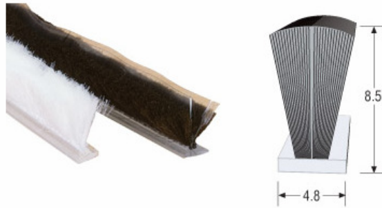
8.5mm weatherpile with fin for use with gaps 3mm to 5.5mm. 4.8mm base.
